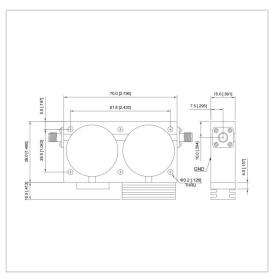
RF Solution offer a wide selection of Dual Junction Isolator for global customers. UIYCDI7048A is a Dual Junction Isolator in Frequency Range of  $200\sim1875$  MHz. It is made of high quality materials under a high standard, the Bandwidth Max of this product is 30%, Insertion Loss Max is  $0.40\sim1.30$  dB and Isolation Min is  $30.0\sim60.0$  dB. The component has a good working performance and stability, it is ideal for handling a Forward Power of 100/300 W.
