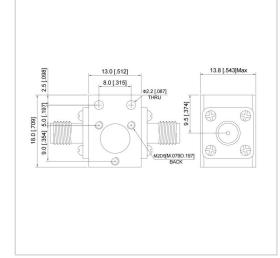
RF Solution offer a wide selection of Coaxial Isolator for global customers. UIYCI1318A is a Coaxial Isolator in Frequency Range of 6.0~35.0 GHz. It is made of high quality materials under a high standard, the Bandwidth Max of this product is 75%, Insertion Loss Max is 0.30~0.60 dB and Isolation Min is 18.0~23.0 dB. The component has a good working performance and stability, it is ideal for handling a Forward Power of 30/60 W.
