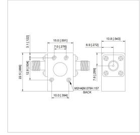
RF Solution offer a wide selection of Coaxial Isolator for global customers. UIYCI1522A is a Coaxial Isolator in Frequency Range of 4.4~7.2 GHz. It is made of high quality materials under a high standard, the Bandwidth Max of this product is 25%, Insertion Loss Max is 0.30~0.50 dB and Isolation Min is 18.0~23.0 dB. The component has a good working performance and stability, it is ideal for handling a Forward Power of 60 W.
