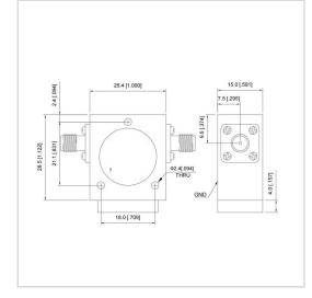
RF Solution offer a wide selection of Coaxial Isolator for global customers. UIYCI2528A is a Coaxial Isolator in Frequency Range of 700~5000 MHz. It is made of high quality materials under a high standard, the Bandwidth Max of this product is 30%, Insertion Loss Max is 0.30~0.50 dB and Isolation Min is 18.0~23.0 dB. The component has a good working performance and stability, it is ideal for handling a Forward Power of 100/150/200 W.
