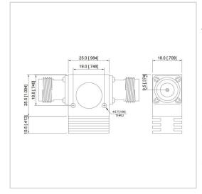
RF Solution offer a wide selection of Coaxial Isolator for global customers. UIYCI2536A is a Coaxial Isolator in Frequency Range of 4.0~8.0 GHz. It is made of high quality materials under a high standard, the Bandwidth Max of this product is 20%, Insertion Loss Max is 0.30~0.50 dB and Isolation Min is 20.0~23.0 dB. The component has a good working performance and stability, it is ideal for handling a Forward Power of 300 W.
