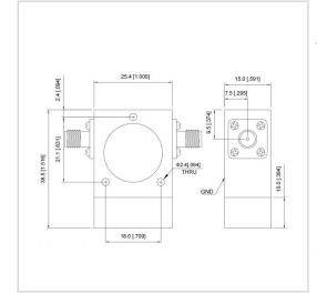
RF Solution offer a wide selection of Coaxial Isolator for global customers. UIYCI2538A is a Coaxial Isolator in Frequency Range of 700~5000 MHz. It is made of high quality materials under a high standard, the Bandwidth Max of this product is 30%, Insertion Loss Max is 0.30~0.50 dB and Isolation Min is 18.0~23.0 dB. The component has a good working performance and stability, it is ideal for handling a Forward Power of 100/150/200 W.
