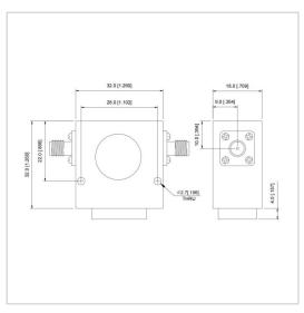
RF Solution offer a wide selection of Coaxial Isolator for global customers. UIYCI3232A is a Coaxial Isolator in Frequency Range of 700~2500 MHz. It is made of high quality materials under a high standard, the Bandwidth Max of this product is 35%, Insertion Loss Max is 0.30~0.50 dB and Isolation Min is 18.0~23.0 dB. The component has a good working performance and stability, it is ideal for handling a Forward Power of 100/200 W.
