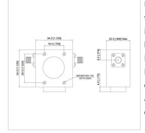
RF Solution offer a wide selection of Coaxial Isolator for global customers. UIYCI3434A is a Coaxial Isolator in Frequency Range of 700~2000 MHz. It is made of high quality materials under a high standard, the Bandwidth Max of this product is 40%, Insertion Loss Max is 0.25~0.6 dB and Isolation Min is 16.0~23.0 dB. The component has a good working performance and stability, it is ideal for handling a Forward Power of 100/200 W.
