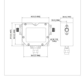
RF Solution offer a wide selection of Coaxial Isolator for global customers. UIYCI4337A is a Coaxial Isolator in Frequency Range of 40.0~50.0 GHz. It is made of high quality materials under a high standard, the Bandwidth Max of this product is 12%, Insertion Loss Max is 0.80~1.60 dB and Isolation Min is 12.0~15.0 dB. The component has a good working performance and stability, it is ideal for handling a Forward Power of 10 W.
