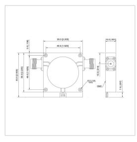
RF Solution offer a wide selection of Coaxial Isolator for global customers. UIYCI5663A is a Coaxial Isolator in Frequency Range of  $130\sim900$  MHz. It is made of high quality materials under a high standard, the Bandwidth Max of this product is 40%, Insertion Loss Max is  $0.30\sim0.70$  dB and Isolation Min is  $16.0\sim23.0$  dB. The component has a good working performance and stability, it is ideal for handling a Forward Power of 100/300 W.
