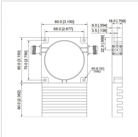
RF Solution offer a wide selection of Coaxial Isolator for global customers. UIYCI80140B is a Coaxial Isolator in Frequency Range of 60~200 MHz. It is made of high quality materials under a high standard, the Bandwidth Max of this product is 20%, Insertion Loss Max is 0.20~1.50 dB and Isolation Min is 16.0~25.0 dB. The component has a good working performance and stability, it is ideal for handling a Forward Power of 500 W.
