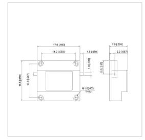
RF Solution offer a wide selection of Dual Junction Isolator for global customers. UIYDDI1716A is a Dual Junction Isolator in Frequency Range of 5.0~25.0 GHz. It is made of high quality materials under a high standard, the Bandwidth Max of this product is 40%, Insertion Loss Max is 0.60~1.20 dB and Isolation Min is 36.0~46.0 dB. The component has a good working performance and stability, it is ideal for handling a Forward Power of 30/65 W.
