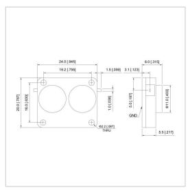
RF Solution offer a wide selection of Dual Junction Isolator for global customers. UIYDDI2420A is a Dual Junction Isolator in Frequency Range of 4.0~7.0 GHz. It is made of high quality materials under a high standard, the Bandwidth Max of this product is 20%, Insertion Loss Max is 0.80~1.00 dB and Isolation Min is 36.0~45.0 dB. The component has a good working performance and stability, it is ideal for handling a Forward Power of 60 W.
