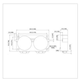
RF Solution offer a wide selection of Dual Junction Isolator for global customers. UIYDDI3819A is a Dual Junction Isolator in Frequency Range of 0.6~5.0 GHz. It is made of high quality materials under a high standard, the Bandwidth Max of this product is 30%, Insertion Loss Max is 0.50~1.20 dB and Isolation Min is 36.0~50.0 dB. The component has a good working performance and stability, it is ideal for handling a Forward Power of 100 W.
