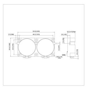
RF Solution offer a wide selection of Dual Junction Isolator for global customers. UIYDDI5025A is a Dual Junction Isolator in Frequency Range of  $200\sim3600$  MHz. It is made of high quality materials under a high standard, the Bandwidth Max of this product is 30%, Insertion Loss Max is  $0.40\sim1.20$  dB and Isolation Min is  $36.0\sim50.0$  dB. The component has a good working performance and stability, it is ideal for handling a Forward Power of 200 W.
