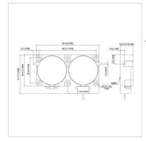
RF Solution offer a wide selection of Dual Junction Isolator for global customers. UIYDDI5031A is a Dual Junction Isolator in Frequency Range of 200~3600 MHz. It is made of high quality materials under a high standard, the Bandwidth Max of this product is 30%, Insertion Loss Max is 0.40~1.20 dB and Isolation Min is 34.0~50.0 dB. The component has a good working performance and stability, it is ideal for handling a Forward Power of 200 W.
