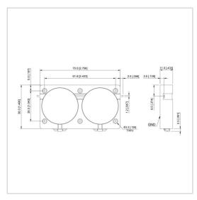
RF Solution offer a wide selection of Dual Junction Isolator for global customers. UIYDDI7038A is a Dual Junction Isolator in Frequency Range of  $200\sim1875$  MHz. It is made of high quality materials under a high standard, the Bandwidth Max of this product is 30%, Insertion Loss Max is  $0.60\sim1.30$  dB and Isolation Min is  $30.0\sim60.0$  dB. The component has a good working performance and stability, it is ideal for handling a Forward Power of 300 W.
