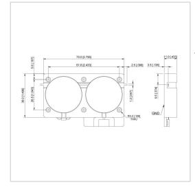
RF Solution offer a wide selection of Dual Junction Isolator for global customers. UIYDDI7046A is a Dual Junction Isolator in Frequency Range of 200~1875 MHz. It is made of high quality materials under a high standard, the Bandwidth Max of this product is 30%, Insertion Loss Max is 0.60~1.30 dB and Isolation Min is 30.0~60.0 dB. The component has a good working performance and stability, it is ideal for handling a Forward Power of 300 W.
