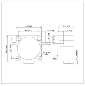
RF Solution offer a wide selection of Drop in Isolator for global customers. UIYDI1212B is a Drop in Isolator in Frequency Range of 0.7~6.0 GHz. It is made of high quality materials under a high standard, the Bandwidth Max of this product is 30%, Insertion Loss Max is 0.30~0.70 dB and Isolation Min is 15.0~23.0 dB. The component has a good working performance and stability, it is ideal for handling a Forward Power of 60 W.
