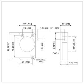
RF Solution offer a wide selection of Drop in Isolator for global customers. UIYDI1220A is a Drop in Isolator in Frequency Range of 4.0~8.0 GHz. It is made of high quality materials under a high standard, the Bandwidth Max of this product is 25%, Insertion Loss Max is 0.25~0.50 dB and Isolation Min is 18.0~23.0 dB. The component has a good working performance and stability, it is ideal for handling a Forward Power of 60 W.
