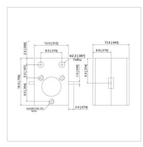
RF Solution offer a wide selection of Drop in Isolator for global customers. UIYDI1318A is a Drop in Isolator in Frequency Range of 17.0~27.5 GHz. It is made of high quality materials under a high standard, the Bandwidth Max of this product is 20%, Insertion Loss Max is 0.50~0.60 dB and Isolation Min is 18.0~20.0 dB. The component has a good working performance and stability, it is ideal for handling a Forward Power of 30 W.
