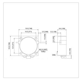
RF Solution offer a wide selection of Drop in Isolator for global customers. UIYDI1919A is a Drop in Isolator in Frequency Range of 600~5000 MHz. It is made of high quality materials under a high standard, the Bandwidth Max of this product is 30%, Insertion Loss Max is 0.25~0.50 dB and Isolation Min is 16.0~25.0 dB. The component has a good working performance and stability, it is ideal for handling a Forward Power of 100 W.
