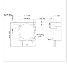
RF Solution offer a wide selection of Drop in Isolator for global customers. UIYDI1925A is a Drop in Isolator in Frequency Range of 0.6~5.0 GHz. It is made of high quality materials under a high standard, the Bandwidth Max of this product is 30%, Insertion Loss Max is 0.25~0.50 dB and Isolation Min is 16.0~25.0 dB. The component has a good working performance and stability, it is ideal for handling a Forward Power of 100 W.
