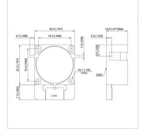
RF Solution offer a wide selection of Drop in Isolator for global customers. UIYDI2027A is a Drop in Isolator in Frequency Range of 400~3000 MHz. It is made of high quality materials under a high standard, the Bandwidth Max of this product is 30%, Insertion Loss Max is 0.25~0.70 dB and Isolation Min is 16.0~25.0 dB. The component has a good working performance and stability, it is ideal for handling a Forward Power of 100 W.
