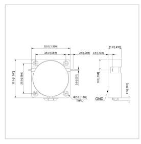
RF Solution offer a wide selection of Drop in Isolator for global customers. UIYDI3232A is a Drop in Isolator in Frequency Range of 0.7~3.1 GHz. It is made of high quality materials under a high standard, the Bandwidth Max of this product is 30%, Insertion Loss Max is 0.20~0.50 dB and Isolation Min is 18.0~23.0 dB. The component has a good working performance and stability, it is ideal for handling a Forward Power of 200 W.
