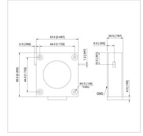
RF Solution offer a wide selection of Drop in Isolator for global customers. UIYDI5356A is a Drop in Isolator in Frequency Range of 300~1500 MHz. It is made of high quality materials under a high standard, the Bandwidth Max of this product is 18%, Insertion Loss Max is 0.20~0.50 dB and Isolation Min is 20.0~25.0 dB. The component has a good working performance and stability, it is ideal for handling a Forward Power of 300/500 W.
