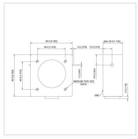
RF Solution offer a wide selection of Drop in Isolator for global customers. UIYDI6060A is a Drop in Isolator in Frequency Range of 45~270 MHz. It is made of high quality materials under a high standard, the Bandwidth Max of this product is 40%, Insertion Loss Max is 0.50~1.80 dB and Isolation Min is 18.0~23.0 dB. The component has a good working performance and stability, it is ideal for handling a Forward Power of 100/200 W.
