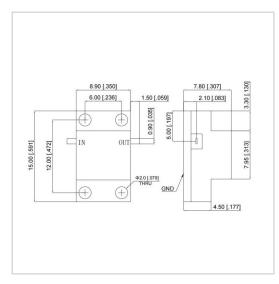
RF Solution offer a wide selection of Drop in Isolator for global customers. UIYDI815A is a Drop in Isolator in Frequency Range of  $5.0\sim30.0$  GHz. It is made of high quality materials under a high standard, the Bandwidth Max of this product is 40%, Insertion Loss Max is  $0.30\sim0.60$  dB and Isolation Min is  $16.0\sim23.0$  dB. The component has a good working performance and stability, it is ideal for handling a Forward Power of 30 W.
