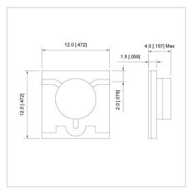
RF Solution offer a wide selection of Microstrip Isolator for global customers. UIYMI1212A is a Microstrip Isolator in Frequency Range of  $3.9\sim5.9$  GHz. It is made of high quality materials under a high standard, the Bandwidth Max of this product is 25%, Insertion Loss Max is  $0.40\sim0.70$  dB and Isolation Min is  $17.0\sim20.0$  dB. The component has a good working performance and stability, it is ideal for handling a Forward Power of 15 W.
