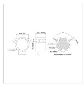
RF Solution offer a wide selection of Surface Mount Isolator for global customers. UIYSI10A is a Surface Mount Isolator in Frequency Range of  $2.4\sim6.0$  GHz. It is made of high quality materials under a high standard, the Bandwidth Max of this product is 20%, Insertion Loss Max is  $0.30\sim0.50$  dB and Isolation Min is  $18.0\sim21.0$  dB. The component has a good working performance and stability, it is ideal for handling a Forward Power of 30 W.
