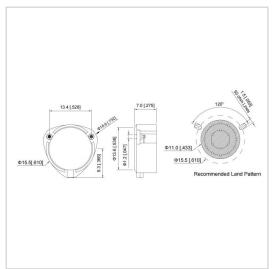
RF Solution offer a wide selection of Surface Mount Isolator for global customers. UIYSI15A is a Surface Mount Isolator in Frequency Range of  $700\sim5000$  MHz. It is made of high quality materials under a high standard, the Bandwidth Max of this product is 15%, Insertion Loss Max is  $0.30\sim0.50$  dB and Isolation Min is  $18.0\sim23.0$  dB. The component has a good working performance and stability, it is ideal for handling a Forward Power of 60 W.
