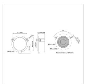
RF Solution offer a wide selection of Surface Mount Isolator for global customers. UIYSI20A is a Surface Mount Isolator in Frequency Range of 400~4200 MHz. It is made of high quality materials under a high standard, the Bandwidth Max of this product is 16%, Insertion Loss Max is 0.25~0.70 dB and Isolation Min is 18.0~25.0 dB. The component has a good working performance and stability, it is ideal for handling a Forward Power of 60 W.
