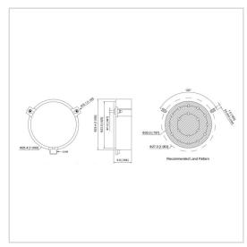
RF Solution offer a wide selection of Surface Mount Isolator for global customers. UIYSI25A is a Surface Mount Isolator in Frequency Range of  $200\sim3600$  MHz. It is made of high quality materials under a high standard, the Bandwidth Max of this product is 30%, Insertion Loss Max is  $0.20\sim0.60$  dB and Isolation Min is  $16.0\sim25.0$  dB. The component has a good working performance and stability, it is ideal for handling a Forward Power of 100 W.
