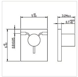
RF Solution offer a wide selection of Microstrip Isolator for global customers. WG0506-07-X-18.0-26.0GHz is a Microstrip Isolator in Frequency Range of 18.0~26.0 GHz. It is made of high quality materials under a high standard, the Insertion Loss Max of this product is 0.60 dB, Isolation Min is 16.0 dB and VSWR Max is 1.40. The component has a good working performance and stability, it is ideal for handling a Forward Power of 4 W.
