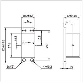
RF Solution offer a wide selection of Drop in Isolator for global customers. WG1017C is a Drop in Isolator in Frequency Range of 17.0~31.0 GHz. It is made of high quality materials under a high standard, the Bandwidth Max of this product is 38%, Insertion Loss Max is 0.80~1.00 dB and Isolation Min is 20.0 dB. The component has a good working performance and stability, it is ideal for handling a Forward Power of 10 W.
