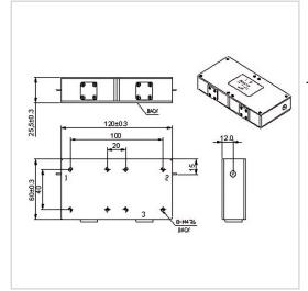
RF Solution offer a wide selection of Dual Junction Isolator for global customers. WG12060H is a Dual Junction Isolator in Frequency Range of 80~230 MHz. It is made of high quality materials under a high standard, the Bandwidth Max of this product is 5~30%, Insertion Loss Max is 0.80~2.20 dB and Isolation Min is 36.0~46.0 dB. The component has a good working performance and stability, it is ideal for handling a Forward Power of 50/100 W.
