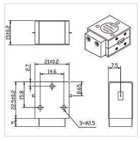
RF Solution offer a wide selection of Drop in Isolator for global customers. WG2123B is a Drop in Isolator in Frequency Range of  $4.0 \sim 8.0$  GHz. It is made of high quality materials under a high standard, the Bandwidth Max of this product is 100%, Insertion Loss Max is  $0.40 \sim 0.60$  dB and Isolation Min is  $18.0 \sim 19.0$  dB. The component has a good working performance and stability, it is ideal for handling a Forward Power of 50 W.
