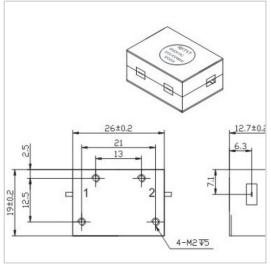
RF Solution offer a wide selection of Dual Junction Isolator for global customers. WG2619C is a Dual Junction Isolator in Frequency Range of 8.0~12.0 GHz. It is made of high quality materials under a high standard, the Bandwidth Max of this product is 100%, Insertion Loss Max is 0.80~1.00 dB and Isolation Min is 20.0~40.0 dB. The component has a good working performance and stability, it is ideal for handling a Forward Power of 30 W.
