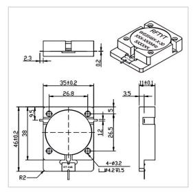
RF Solution offer a wide selection of Drop in Isolator for global customers. WG3546X-100W is a Drop in Isolator in Frequency Range of  $300\sim1850$  MHz. It is made of high quality materials under a high standard, the Bandwidth Max of this product is 30%, Insertion Loss Max is  $0.20\sim0.80$  dB and Isolation Min is  $16.0\sim25.0$  dB. The component has a good working performance and stability, it is ideal for handling a Forward Power of 100 W.
