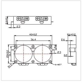
RF Solution offer a wide selection of Dual Junction Isolator for global customers. WG4020X is a Dual Junction Isolator in Frequency Range of  $700\sim2700$  MHz. It is made of high quality materials under a high standard, the Bandwidth Max of this product is  $5\sim20\%$ , Insertion Loss Max is  $0.60\sim1.20$  dB and Isolation Min is  $36.0\sim46.0$  dB. The component has a good working performance and stability, it is ideal for handling a Forward Power of 100 W.
