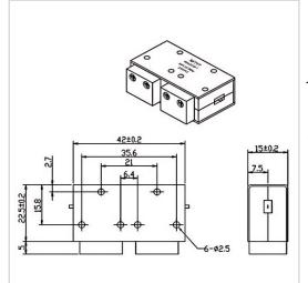
RF Solution offer a wide selection of Dual Junction Isolator for global customers. WG4223B is a Dual Junction Isolator in Frequency Range of 4.0~8.0 GHz. It is made of high quality materials under a high standard, the Bandwidth Max of this product is 100%, Insertion Loss Max is 0.80~1.20 dB and Isolation Min is 36.0~38.0 dB. The component has a good working performance and stability, it is ideal for handling a Forward Power of 50 W.
