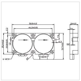
RF Solution offer a wide selection of Dual Junction Isolator for global customers. WG5025X is a Dual Junction Isolator in Frequency Range of  $350\sim4300$  MHz. It is made of high quality materials under a high standard, the Bandwidth Max of this product is  $5\sim15\%$ , Insertion Loss Max is  $0.40\sim1.40$  dB and Isolation Min is  $34.0\sim50.0$  dB. The component has a good working performance and stability, it is ideal for handling a Forward Power of 200 W.
