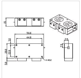
RF Solution offer a wide selection of Dual Junction Isolator for global customers. WG5028C is a Dual Junction Isolator in Frequency Range of  $3.0\sim6.0$  GHz. It is made of high quality materials under a high standard, the Bandwidth Max of this product is 100%, Insertion Loss Max is  $0.60\sim1.60$  dB and Isolation Min is  $36.0\sim38.0$  dB. The component has a good working performance and stability, it is ideal for handling a Forward Power of 100 W.
