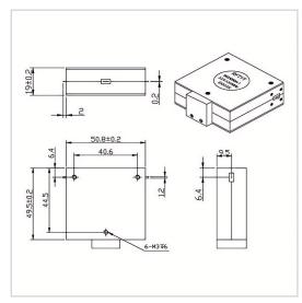
RF Solution offer a wide selection of Drop in Isolator for global customers. WG5050A is a Drop in Isolator in Frequency Range of 1.35~3.0 GHz. It is made of high quality materials under a high standard, the Bandwidth Max of this product is 100%, Insertion Loss Max is 0.50~0.80 dB and Isolation Min is 16.0~18.0 dB. The component has a good working performance and stability, it is ideal for handling a Forward Power of 150 W.
