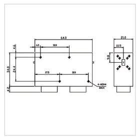
RF Solution offer a wide selection of Dual Junction Isolator for global customers. WG6434A is a Dual Junction Isolator in Frequency Range of  $2.0\sim4.0$  GHz. It is made of high quality materials under a high standard, the Bandwidth Max of this product is 100%, Insertion Loss Max is  $1.00\sim1.20$  dB and Isolation Min is  $36.0\sim38.0$  dB. The component has a good working performance and stability, it is ideal for handling a Forward Power of 100 W.
