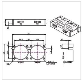
RF Solution offer a wide selection of Dual Junction Isolator for global customers. WG7038X is a Dual Junction Isolator in Frequency Range of  $400\sim1850$  MHz. It is made of high quality materials under a high standard, the Bandwidth Max of this product is  $5\sim20\%$ , Insertion Loss Max is  $0.40\sim1.40$  dB and Isolation Min is  $32.0\sim50.0$  dB. The component has a good working performance and stability, it is ideal for handling a Forward Power of 100~W.
