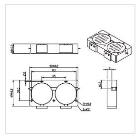
RF Solution offer a wide selection of Dual Junction Isolator for global customers. WG9050X is a Dual Junction Isolator in Frequency Range of  $300\sim1250$  MHz. It is made of high quality materials under a high standard, the Bandwidth Max of this product is  $5\sim20\%$ , Insertion Loss Max is  $0.60\sim1.60$  dB and Isolation Min is  $30.0\sim50.0$  dB. The component has a good working performance and stability, it is ideal for handling a Forward Power of 100~W.
