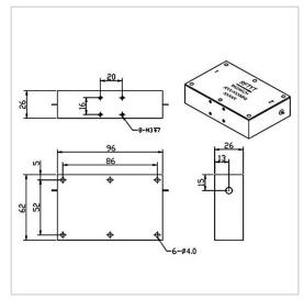
RF Solution offer a wide selection of Dual Junction Isolator for global customers. WG9662H is a Dual Junction Isolator in Frequency Range of  $300\sim1250$  MHz. It is made of high quality materials under a high standard, the Bandwidth Max of this product is  $5\sim20\%$ , Insertion Loss Max is  $0.60\sim1.60$  dB and Isolation Min is  $32.0\sim50.0$  dB. The component has a good working performance and stability, it is ideal for handling a Forward Power of 100~%.
