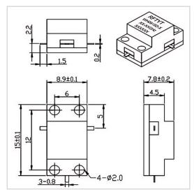
RF Solution offer a wide selection of Drop in Circulator for global customers. WH0915D is a Drop in Circulator in Frequency Range of  $6.0\sim10.0$  GHz. It is made of high quality materials under a high standard, the Bandwidth Max of this product is 50%, Insertion Loss Max is  $0.30\sim0.60$  dB and Isolation Min is  $18.0\sim23.0$  dB. The component has a good working performance and stability, it is ideal for handling a Power of 30 W.
