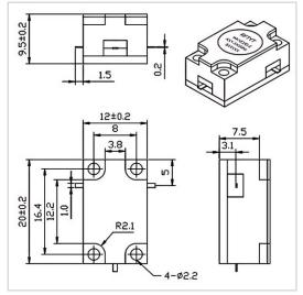
RF Solution offer a wide selection of Drop in Circulator for global customers. WH1220D is a Drop in Circulator in Frequency Range of 5.5~7.0 GHz. It is made of high quality materials under a high standard, the Bandwidth Max of this product is 60%, Insertion Loss Max is 0.30~0.50 dB and Isolation Min is 18.0~23.0 dB. The component has a good working performance and stability, it is ideal for handling a Power of 30 W.
